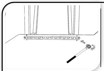
Slide a second washer (J) inside the ceiling rail (H) and line up with the second correct slot.
