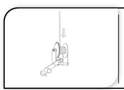
Wind the lifting cable (F) onto the winch spool (D) using either the winch handle (E) or power drill (T).
