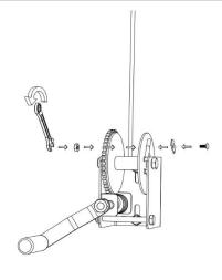
Place the cable clamp -- included with the winch (D) – over the end of the lifting cable (F) and tighten the nut onto the bolt with the 10mm wrench (Z).
