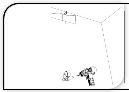
Drill two 3/16" pilot holes at the locations marked in Step 14 with the drill (T) and drill bit (U).
