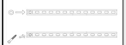
Slide one washer (J) inside the ceiling rail (H) and line up with the correct slot found in Step 5.
