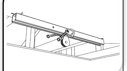
Tighten the nut (L) onto the bolt (L) using two 9/16" wrenches (Y).
