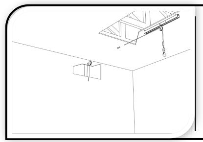
Feed the lifting cable (F) through the ceiling mount pulley (K) toward the corner mount pulley (M).
