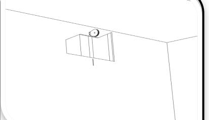
Install the corner mount pulley (M) using the drill (T), 1/4" square drive (G) and the four self-starting wood screws (N).
