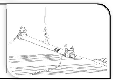
Marker sewn into strap at 21" to achieve correct balance (both straps)
