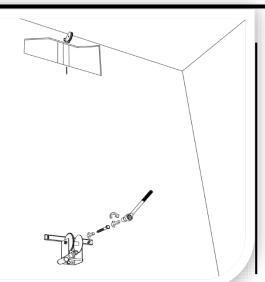
Place the bubble level (AA) on the top edge of the winch (D).
