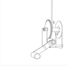
Feed the lifting cable (F) down the back side of the winch spool (D).
