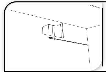
Measure from an adjacent wall to the center of the wall stud measured in Step 2.
